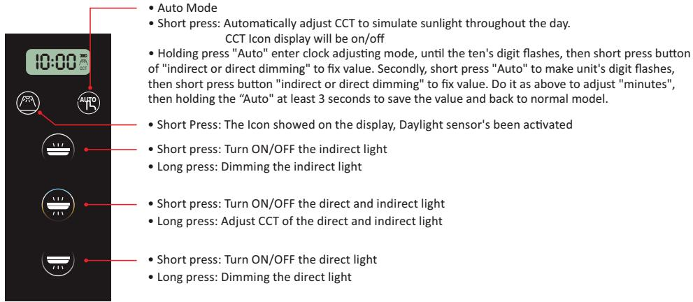
Remark: When dim the light or adjust CCT to Max/Min level, the green indicator will flash for three times.
