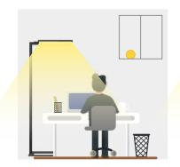
The lamp brightness reduce to 30% after 20min when no motion is detected
