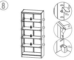
Before placing shelves, place four shelves holder into perforated slots at the same height for each shelf location.
