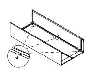
Align and attach the right side panel to the back panels at right angles and tighten with 3 screws at the 3 indicated locations.
