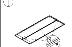
Align and attach the left back panel to the right back panel with 3 screws and nuts securely.
