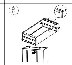
Attach the top panel to the top of the cabinet frame and secured with seven screws.
