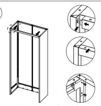
Attach the top bracket to the side panels and tighten with two screws, each side (totally four screws).
