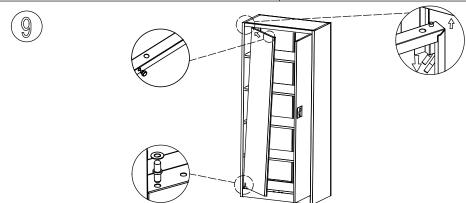
Install bottom hinge pin and washer on each side of the bottom bracket .Make sure thewasher is on the bottom hinge pin .Lower the left door onto bottom left bottom hinge pin, then swing the left door into top panel while pulling down on the latch, align latch with hole in top panel and release when latch is inposition.Repeat above step for right door insert key into lock to verify proper operation.
