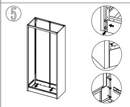
Attach the bottom bracket to the side panels and tighten with three screws each side(totally six screws).
