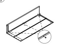
Align and attach the left side panel to the back panels at right angles and tighten with 3 screws at the 3 indicated locations.
