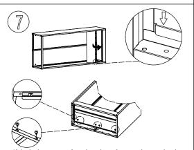
Slide the bottom panel to the cabinet frame and secured with four screws on the bottom, Makesure the notch on the edge of bottom panel face forward.
