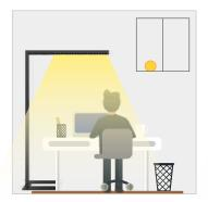
The lamp brightness reduce to 30% after 20min when no motion is detected
